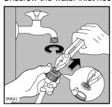
Remove and clean the filters using a hard bristle brush. Replace the filters and tighten up the inlet hoses.
